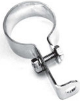
Sportster® Front Pipe Clamp Replaces OEM 65514-58. Use on all 1958-78 XL's. Also can be used as a universal hanger. Chrome plated. Sold each. 1436
