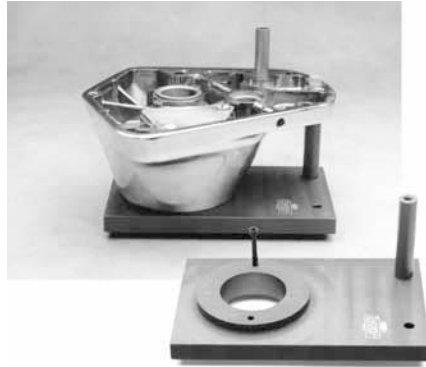
Jims Cam Cover Holding Tool Use tool to hold cam cover for removing and installing bushings. Clamps in vice or mill. Holds cam cover flat and keeps it from being scratched. 31423 BT 1970-99 (1041-TC)
