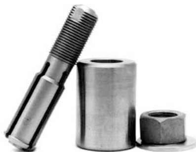
Cam Bearing Puller Used to remove inner cam bearing, caged Torrington, without splitting cases while preventing rollers from coming out during removal. 31411 BT 1958-99 (95760-TB) (Jims) 26057 BT 1958-99 (Preston)
