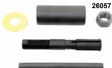
Cam Bearing Puller Used to remove inner cam bearing, caged Torrington, without splitting cases while preventing rollers from coming out during removal. 31411 BT 1958-99 (95760-TB) (Jims) 26057 BT 1958-99 (Preston)
