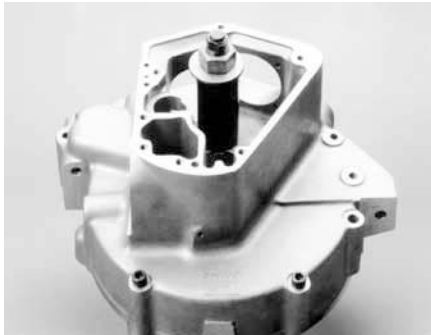
Jims Cam Bearing Installer Use tool for inner Torrington bearings 9058 on BT 1958-99 models. 31535
