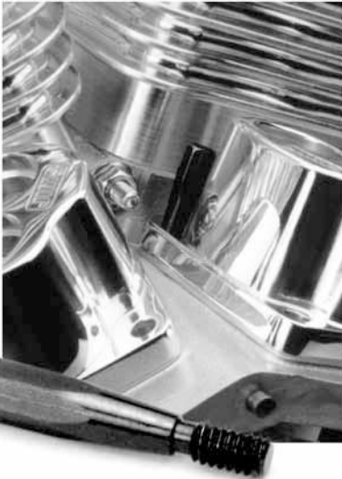
Jims Late Shovel and Evo Tappet Block Alignment Tool Use to align oil hole from crankcase to tappet block. Using two will allow alignment of rocker boxes on Evo heads. 31440 BT Late 1977-on single cam including aftermarket and S&S motors (1/4-20 threads)
