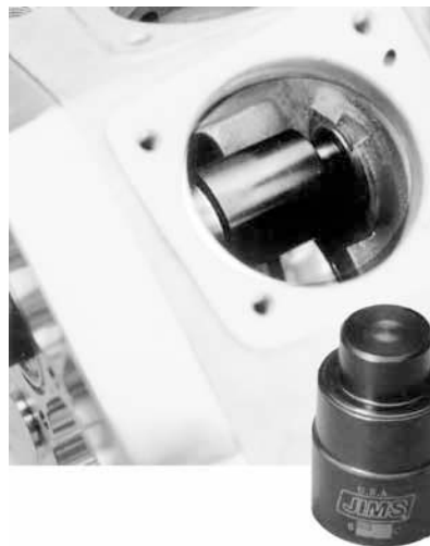
Jims Cam Bearing Gauge Use pins to check if your cam is too tight or too loose. A tight cam can eat up the end of the journal and cause other problems. A loose cam can be noisy and cause cam, bearing and roller wear. 31485 BT 1958-on single cam only all aftermarket and S&S motors 31486 XL 1957-90
