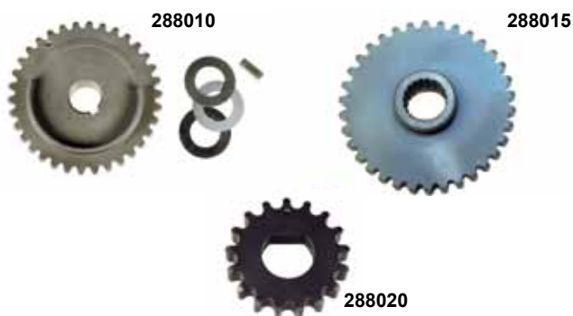
Andrews TC 88 Rear Cam Sprocket Kit 99-06 All Andrews Twin 88 cam kits require a heat treated 34T rear cam drive sprocket that replaces OEM 25563-99. Sprockets are made from heat treated alloy steel and are longer than stock providing greater stability. Includes a full length 3/16 drive key and 3 spacer shims that allow the installed length of new sprocket to be the same as the original stock sprocket plus spacer.
