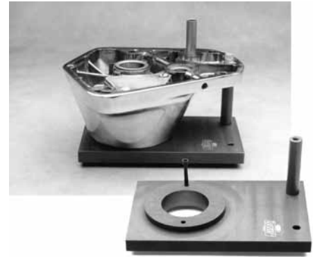
Jims Cam Cover Holding Tool Use tool to hold cam cover for removing and installing bushings. Clamps in vice or mill. Holds cam cover flat and keeps it from being scratched. 31423 BT 1970-99 (1041-TC)
