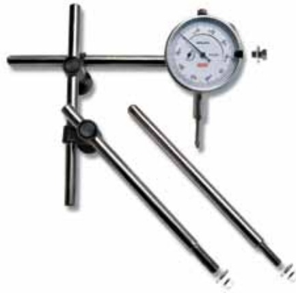
Jims End Play Gauge Indicator Tool Features H-D thread pitch for mounting to cases when checking end play on engines or transmissions. Comes with 1/4"-20 and 5/16"-18 threads on the mounting rod. Can be used in any position for checking cam, shift drum, rocker or breather gear end play, as well as fly-wheel, mainshaft, or starter gear runout. For use on all Big Twin and Sportster. 31540
